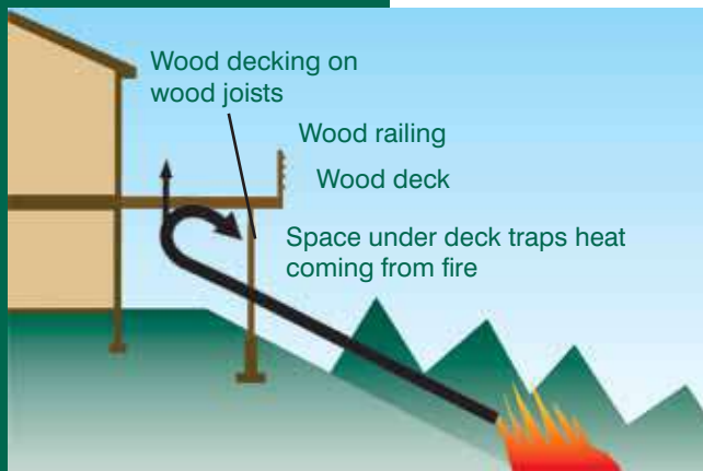
Figure 4-10: Conventional deck in a fire
